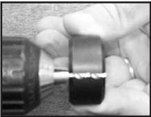
Step 2 -The *Drill Bit* needs to be set so that 3/4 " is protruding beyond the chuck jaws. An easy way to accomplish this is to use the Staking Cap as a setting gage, see illustration .
